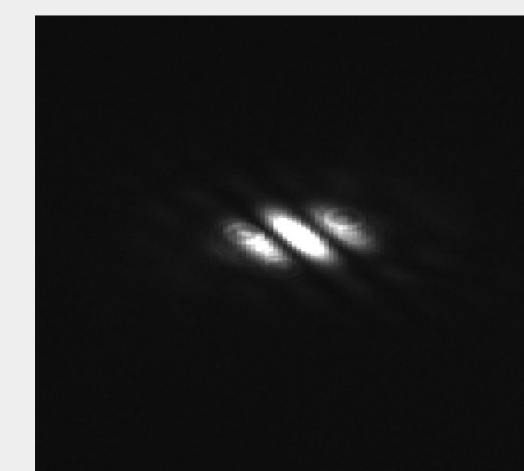
Figure 10. Pixelink image showing S6 properly aligned with S0. Strong interference bands indicate proper alignment.
