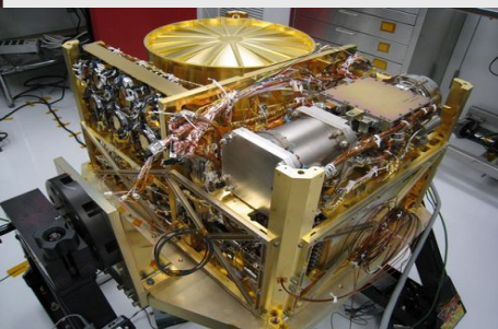
Figure 1. Sample Analysis at Mars (SAM). SAM consists of a GCMS that allows for identification of organics potentially discovered on Mars.
